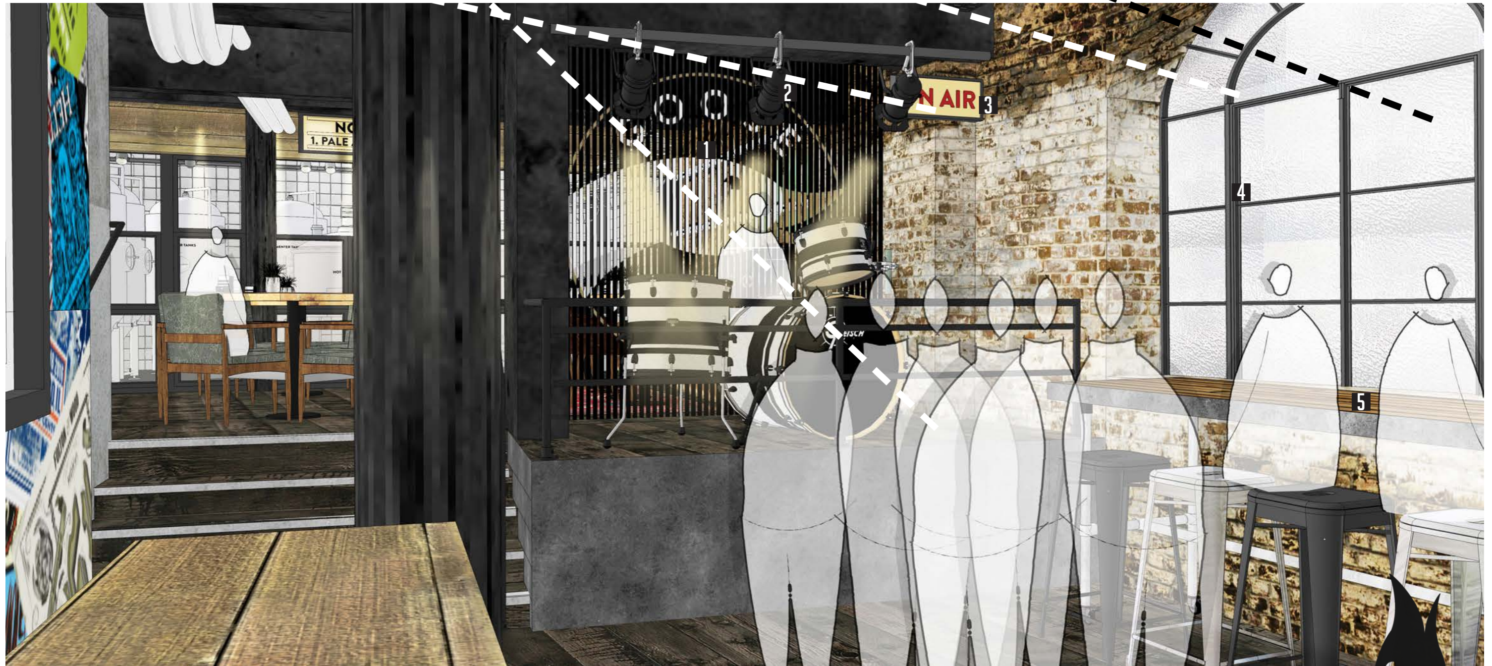
1- Printed chain screen that extends out during performances with full Goose Island logo 2- Stage lighting rig to illuminate performers 3- Illuminated 'On Air' sign wall mounted to indicate when bands are playing 4- Opening up the arched windows and replacing the glass with a muffled distorted glass with a crittall style hardwood frame 5- Kee klamp movable tables run in a line along wall when bands are playing to open up the space and still provide areas for seating
