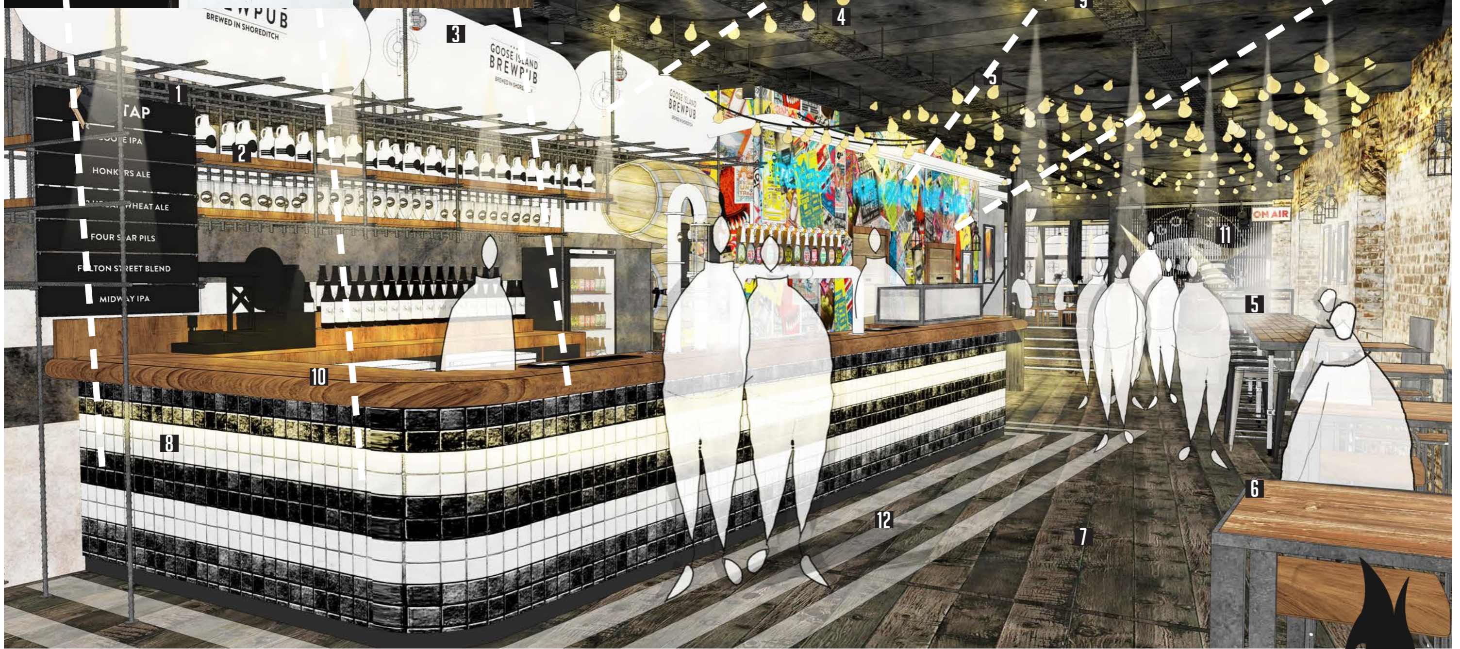
1- Chalkboard menus fixed on hooks to back-bar framework 2- Welded rebar back-bar display with stained oak illuminated shelves 3- Stainless steel beer kegs suspended from soffit with exposed stainless steel beer pipes 4- Existing soffit to be retained and sprayed out black to add atmosphere 5- Festoon lights at 2200k to be suspended along run of bar to add some atmospheric glow and interest to the ceiling 6- Folding tables that form small beer shelf tables when folded and long 5 top tables when extended (see detail) 7- Sand and re-stain the existing hardwood floor 8- Black and white crackle glaze tiles to represent the Chicago state flag 9- Spray out services and cable tray 10- Stained oak bar top with under counter LED to wash down the tiles 11- Printed chain screen that extends out during performances 12- Painted white stripes on floor which will fade and age over time
